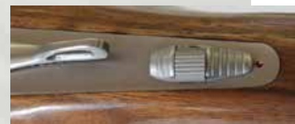
The safety catch-cum-barrel selector is in a traditional position.
