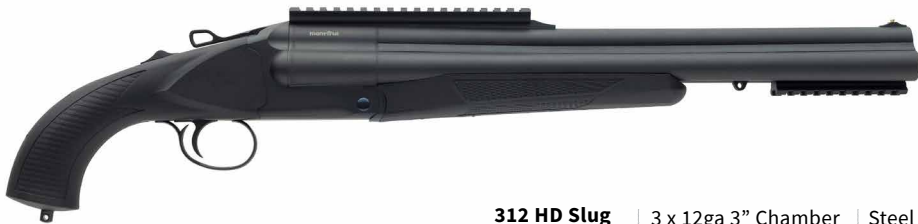
312 HD Slug K31222 3 x 12ga 3" Chamber 47cm Barrel Fixed Cyl Picatinny rails Steel receiver Manual safety Extractor Pistol Grip 3.35 kg
